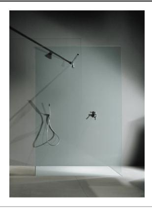
Fixed shower panel with horizontal support element. Crystal glass wall, 10 mm (3/8) thick, 2200 mm (86" 5/8) high. Define in the order: dimensions A and B, where A is always the entrance and the glass variant and add the specific charge. Construction work is required to recess the floor profiles if desired. However, they can also be mounted with screws and anchors, if installed on a finished floor.
