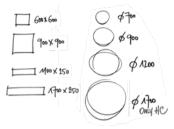
The 48V Superloop comes in different kind of shapes and dimensions, perfect to fit any type of project. Square versions in 600mm by 600mm or 900mm by 900mm, rectangular versions in 1100mm or 1700mm by 250mm or – similar to the SBL version – circular Superloops with diameters from 700mm up to 1700mm, all of them seamlessly welded together to avoid any visual joints.
