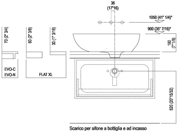
Drain for bottle trap and concealed waste trap
