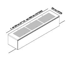
Note: Upon request, and after technical evaluation, other Corian® colours and types of marble are possible. It is available with a minimum length of 80 cm (31 $^{\circ}$  1/4) and a maximum length of 260 cm (102 $^{\circ}$  23/64).
