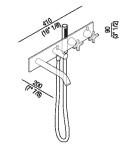
Built in thermostatic bathtub tap unit with flow deviator and handheld shower holder. Finished items to complete with shower heads, flexible hoses and handheld showers.
