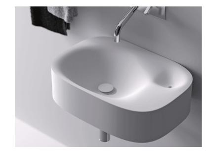
Wall mounted washbasin in white Cristalplant® biobased with overflow hole in a small basin connected with the main basin, which also can be used as a soap holder. Wall mounted version with or without tap hole. Designed for waste .MET0563. Fixing kit included. The overflow hole has a maximum capacity of 8 l/min, therefore it is advisable to install a waste designed for washbasins without overflow.
