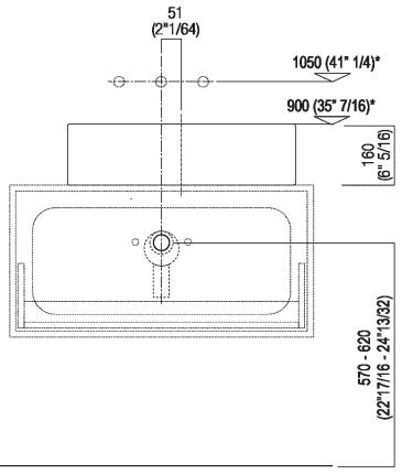
Scarico per sifone a bottiglia e ad incasso Drain for bottle trap and concealed waste trap
