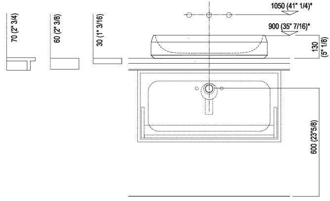
Scarico per sifone a bottiglia e ad incasso Drain for bottle trap and concealed waste trap
